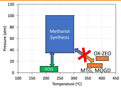
**Similar process conditions offer the opportunity** for process intensification to enable direct syngas-to-fuels through methanol **in a single reactor**
