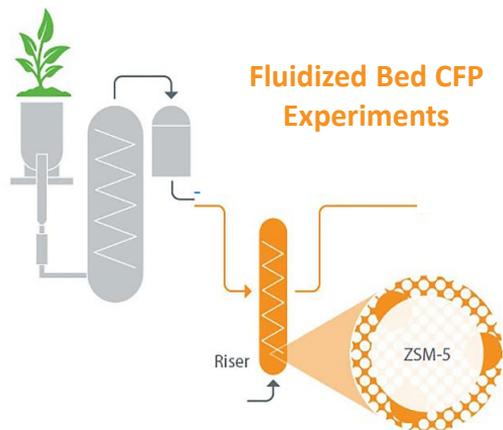
**Approach:** Develop modified zeolites with Johnson Matthey that target biomass conversion and are compatible with refinery fluidized catalytic cracking (FCC) catalysts; prepare CFP oils using a coupled pyrolyzer/FCC plant; evaluate catalyst impact on oil composition; assess FCC co-processability to biogenic carbon containing fuels.
