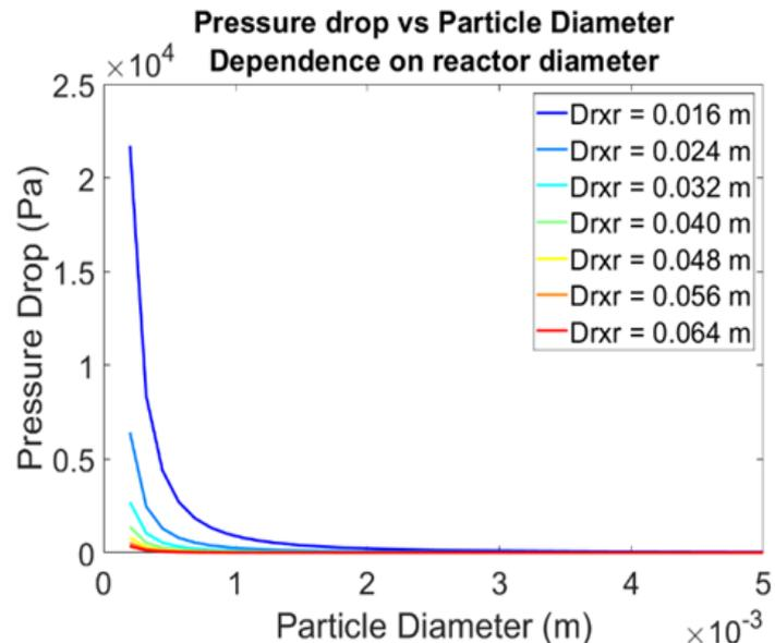
Utilizing smaller  $\text{TiO}_2$  supports improves deoxygenation performance but increases pressure drop and necessitates the use of low L/D reactors with limited heat transfer capabilities
