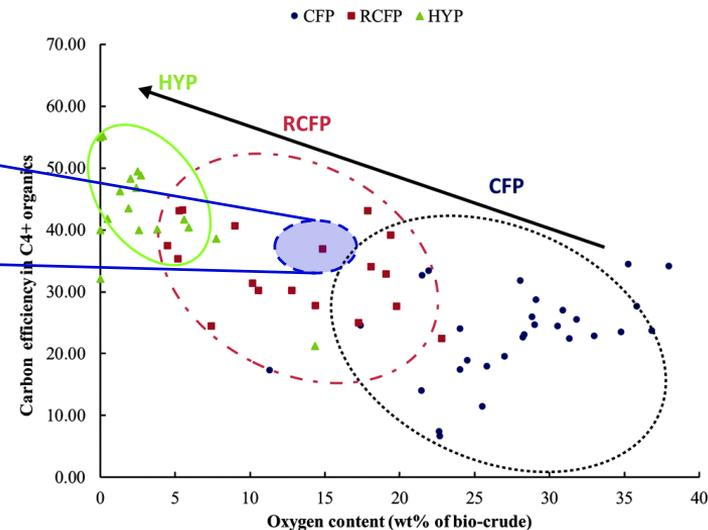
*Data are consistent with literature benchmarks performed under hydrodeoxygenation conditions*
