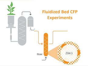
**Approach:** Develop modified zeolites with Johnson Matthey that target biomass conversion and are compatible with refinery fluidized catalytic cracking (FCC) catalysts; prepare CFP oils using a coupled pyrolyzer/FCC plant; evaluate catalyst impact on oil composition; assess FCC co-processability to biogenic carbon containing fuels.
