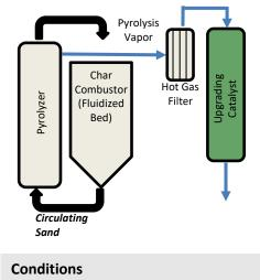
Feedstock: Loblolly Pine Catalyst: 0.5 wt% Pt/TiO<sub>2</sub> Pyrolysis Temperature: 500 °C Upgrading Temperature: 435 °C Catalyst Mass: 100 g WHSV: 1.4 g biomass/gcat\*h Near Atmospheric Pressure Hydrogen Concentration: 83% Biomass:Catalyst Ratio: 3-12 **Progress:** reducing the size of the catalyst support reveals potential for improved deoxygenation activity and increased cycle length
