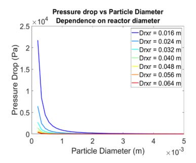
Utilizing smaller TiO<sub>2</sub> supports improves deoxygenation performance but increases pressure drop and necessitates the use of low L/D reactors with limited heat transfer capabilities
