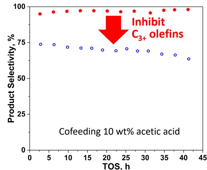
Cu/H-ZSM-5, 250 °C, 1.0 h<sup>-1</sup>, 0.22 mL/h liquid flow, 30 cm<sup>3</sup>/min H<sub>2</sub>, BDO conversion 97-100%
