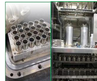
Multi-batch and 1.4 mL Fixed-Bed Flow Reactors
