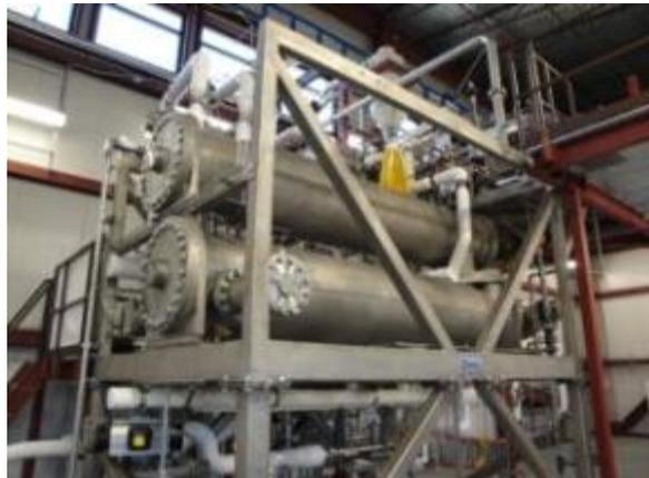
Whole slurry enzymatic hydrolysis in 130 L high-solids at 20% solids (>130 g/L monomer sugar), 40 L of slurry stored
