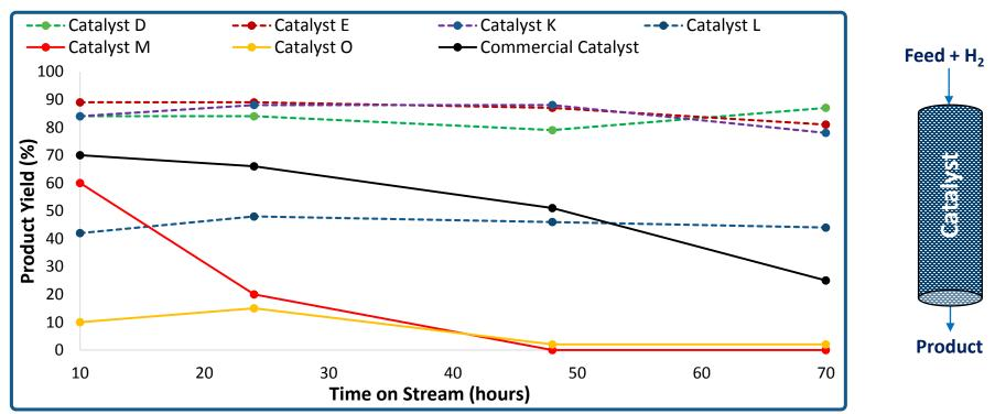
Flow experiments at 150°C (commercial catalyst at 180°C), 12.6 Mpa,  $H_2$  to feed ratio of 15.5 and weight hourly space velocity of 0.8 hr<sup>-1</sup>
