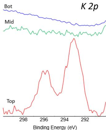
XPS data confirms K deposition on the leading edge of the catalyst bed. (ACSC)
