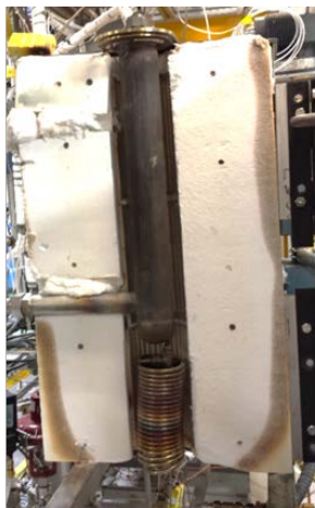
Bubbling fluidized bed reactor at NREL for biomass fast pyrolysis experiments.
